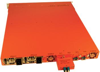
Hardware filters based on any pattern in the GigaVUE 420 header may be enabled to eliminate unwanted packets. The system can be managed remotely by telnet or SSH2, and authenticated with TACAC+ or RADIUS.
