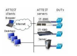
Figure 1. ATTEST supports a flexible, distributed test environment
